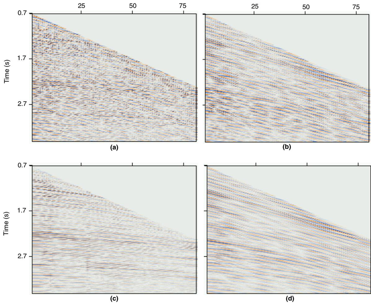
**Figure 3. Vector wavefield separation for an OBC common receiver gather: (a) vertical component, (b) inline component, (c) P wave recovered via PIM, and (d) P-S wave recovered via PIM. The shot interval is 25 m, with source-receiver offsets here ranging from 693 m to 2668 m. The sample interval is 2 ms.**
