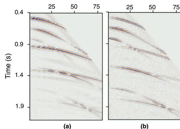
**Figure 1. Two-component synthetic dataset: (a) vertical component, and (b) inline component. Trace spacing is 30m. Signal bandwidth is 12-90Hz. True relative amplitudes are shown.**
