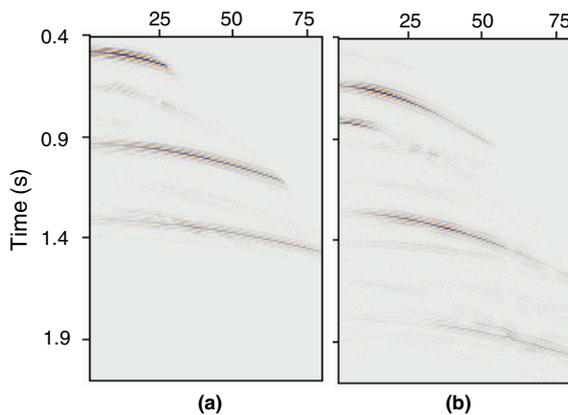
**Figure 2.** Wavefields recovered from synthetic data shown in Figure 1 via PIM: (a) P wave, and (b) P-S wave. Initial parameter estimates for PIM were recovered directly from the seismic data and single-trace polarisation analysis. True relative amplitudes are shown.
