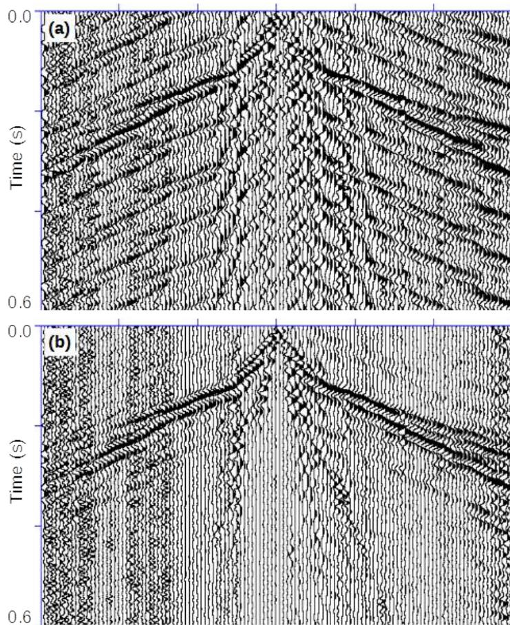
Figure 4: Removal of correlation noise via digital filtering. (a) Mini-SOSIE record generated from an impact sequence having poor randomness. (b) If the impact sequence is well known much of the correlation noise can be removed using digital filters.
