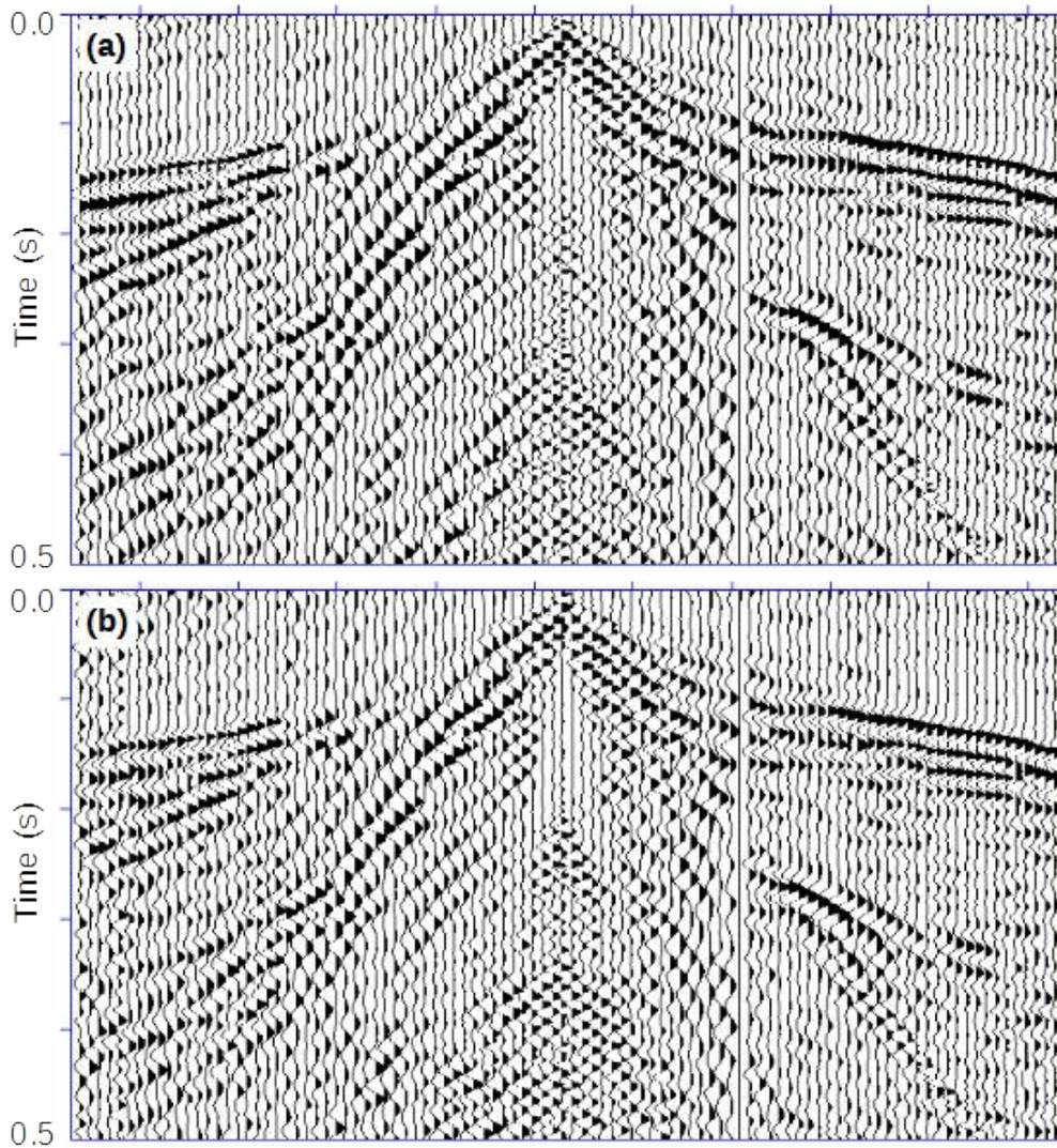
Figure 1: Comparison of a shallow Mini-SOSIE record acquired with (a) typical ram count (250) and (b) with reduced ram count (100). In this case, the larger ram count provides only a small improvement in quality.
