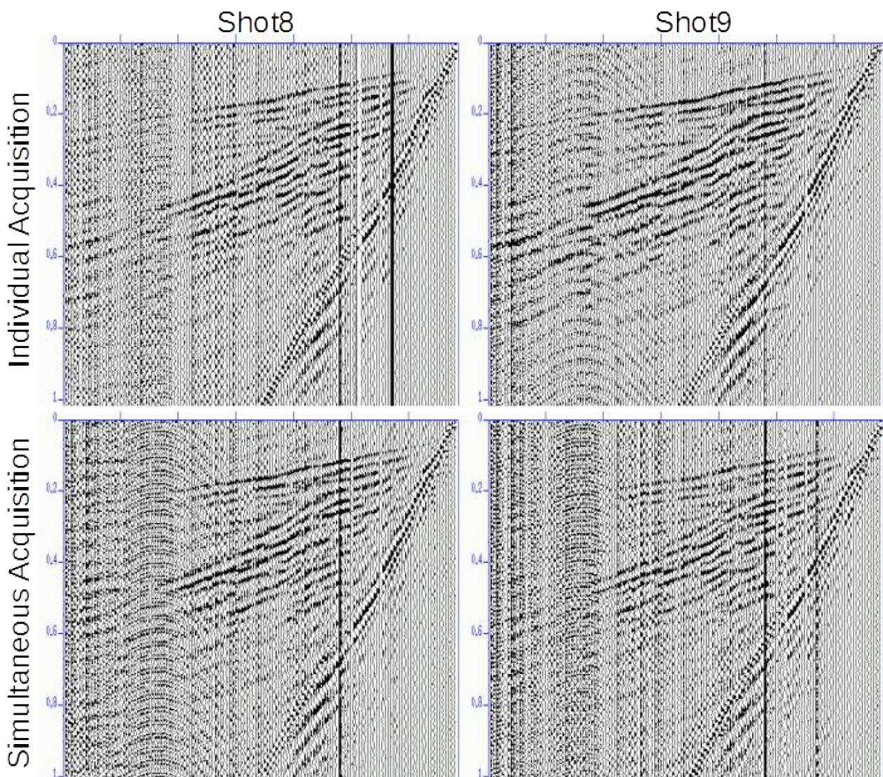
Figure 6: Comparison of individual and simultaneous acquisition for adjacent shot points.
