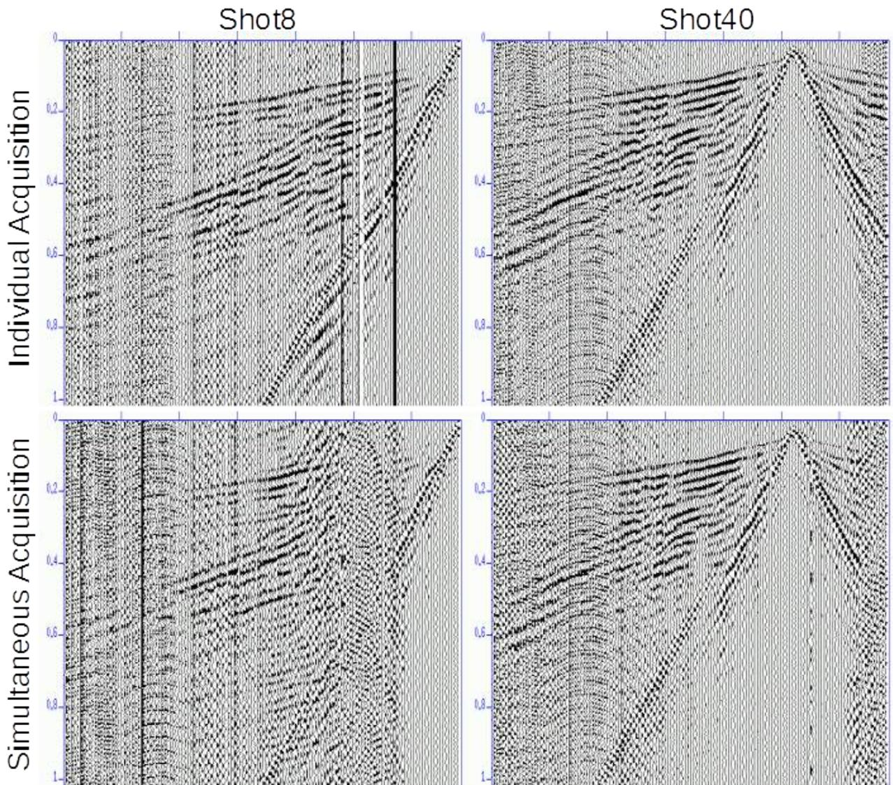
Figure 7: Comparison of individual and simultaneous acquisition for separated shot points.
