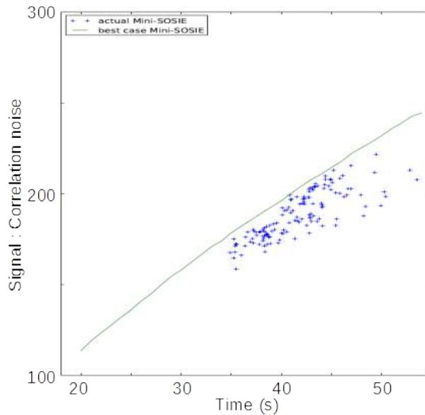
Figure 3: Examination of relationship between signal, correlation noise, and recording time for typical system limitations (0.5ms sample rate, max impact rate approximately 10Hz, 300 rams). Green line indicates the best possible theoretical result, blue dots are based on actual impact sequences from field recordings. As acquisition time is reduced (i.e. ram rate increased), signal/noise ratio reduces. From Fletcher (2012).
