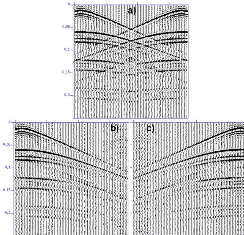
Figure 5: Model example of simultaneous Mini-SOSIE acquisition. (a) two impacts acquired at different locations at the same time interfere. (b) and (c) records obtained by correlation of a combined Mini-SOSIE record from two sources with individual impact sequences. There is some cross contamination on far offsets.
