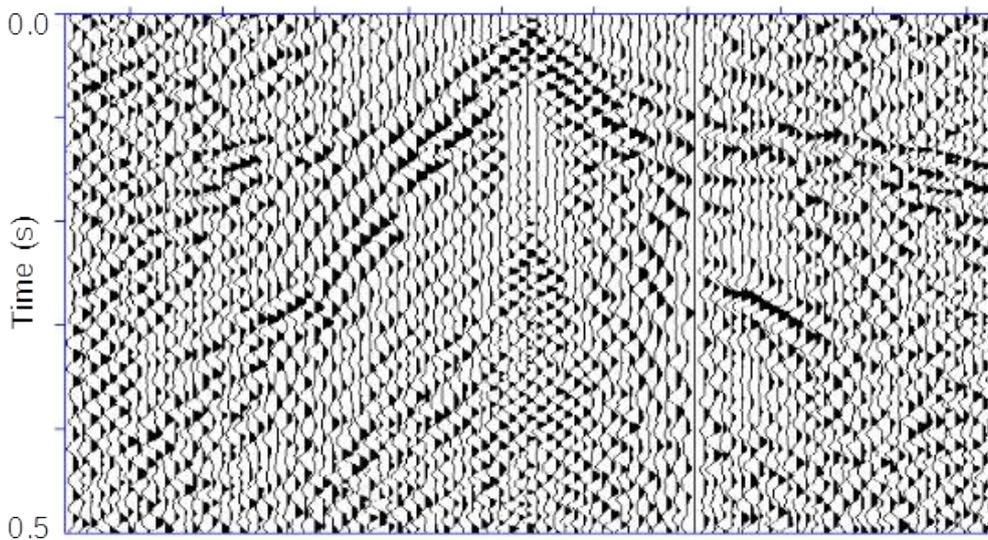
Figure 2: A reduced ram count (150) in the presence of strong noise sources may result in significantly reduced signal-to-noise ratio. Effectiveness of reduced ram counts need to be assessed based on the site noise conditions.
