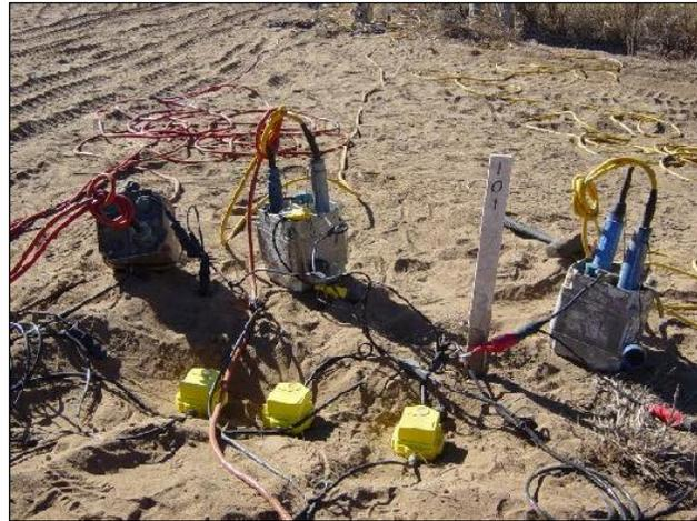
**Figure 7.1 Field acquisition of Trial Dataset #3: planting 3C geophones (left); and a 3C receiver station (above).**
