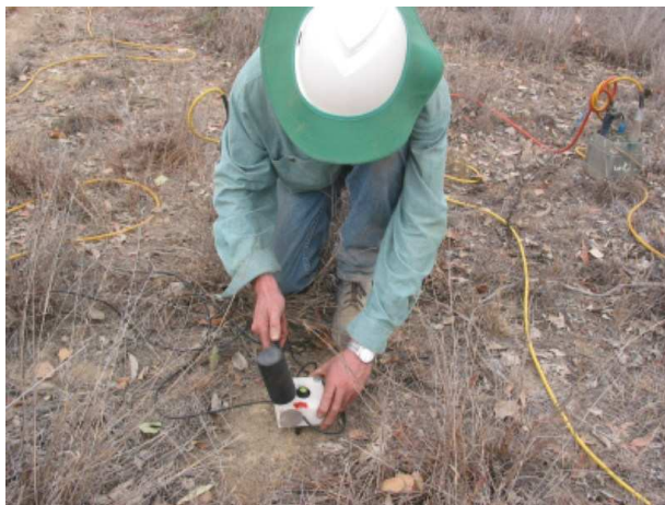
Figure 2.2 Planting of the multi-component geophones requires accurate alignment in both the vertical and horizontal sense to ensure optimum acquisition of both P and PS waves. Geophones are planted firmly using a shock-proof hammer following removal of any loose top soil. Bull's eye spirit levels are used to ensure correct vertical orientation.
