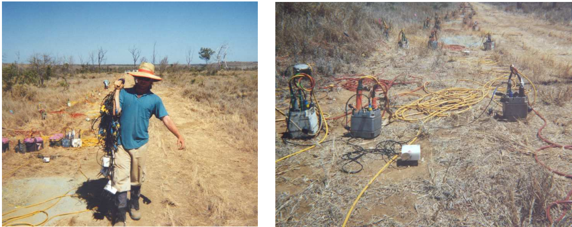
Figure 4.1 Field acquisition of Trial Dataset #1 – laying out recording equipment (left) and a three-component receiver station (right).
