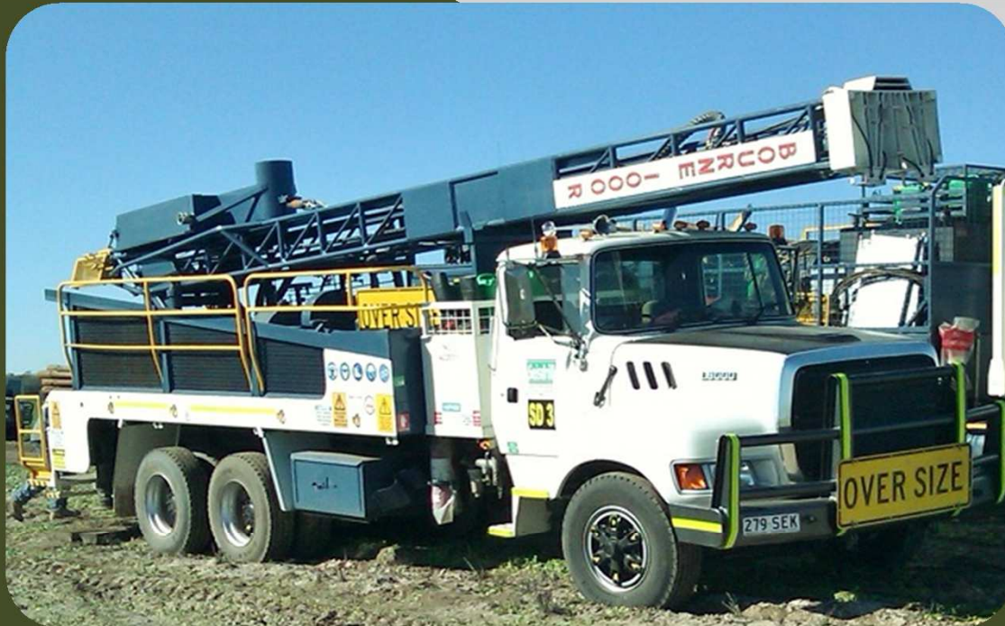
Ford Louisville L8000 with mounted drill rig
