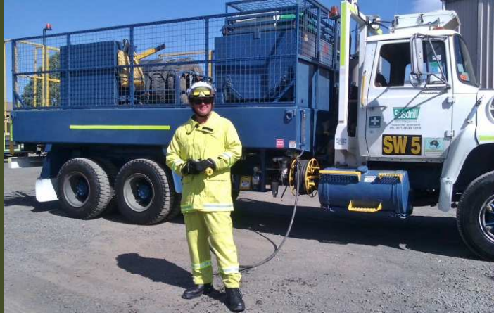
Water Truck set up as Fire Support
