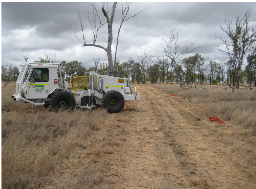
Figure 3.5: Envirovibe moving along a source line at an angle to a receiver line. Communication cable is visible running along the receiver line.
