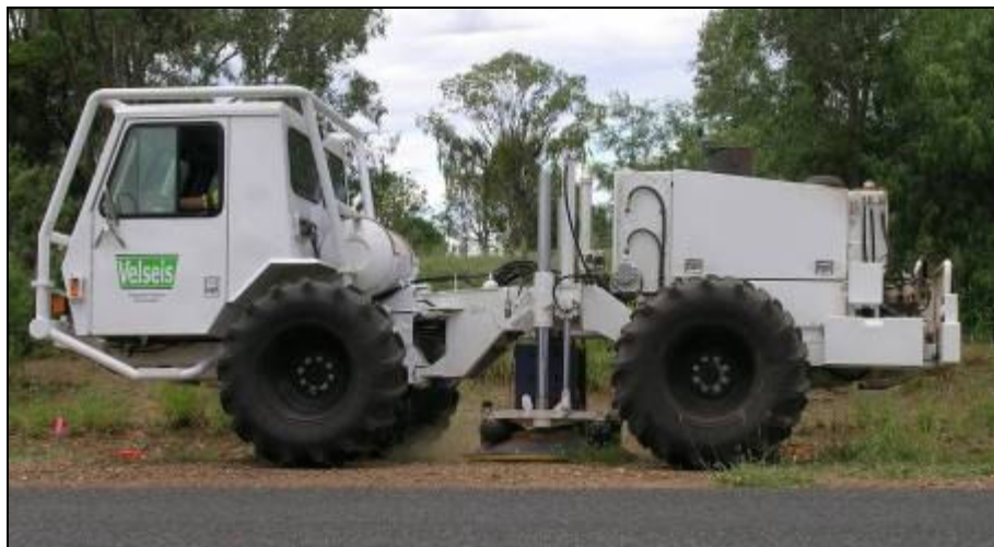
Figure 1: Envirovibe mounted on IVI Minibuggy.
